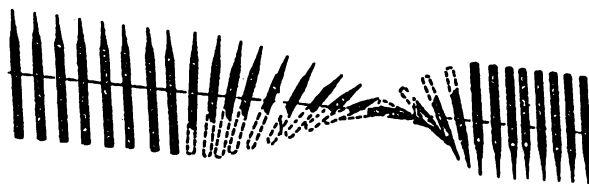
Figure 2. Scheme of two domains separated by a Bloch wall.
